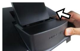
5.5 Tilt the screen up or down to your desired angle. Please do not press on the LCD panel while setting up the tilt angle.
