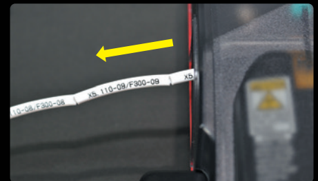
LETATWIN prints and half cut the tubing.
