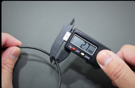
Check the outer wire diameter.
